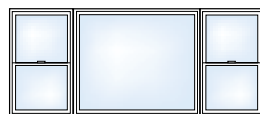
A Picture window mullered with two Single Hung windows. Picture windows may be substituted for Single Hung windows.
