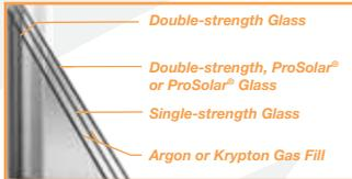
This package features a 1" insulating glass unit with three panes of double-strength glass that produce two separate air spaces for added insulation. Combine this with two layers of ProSolar or ProSolar Shade double-strength glass, Super Spacer and Argon or a heavier Krypton gas fill to achieve superior thermal performance.
