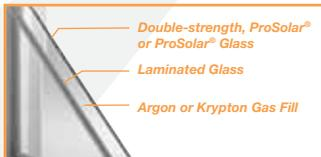
For the ultimate combination of energy efficiency and security, this remarkable glass package features a 1" I.G. unit with laminated glass and a layer of ProSolar or ProSolar Shade double-strength glass. Add an Argon or Krypton gas fill along with the Super
