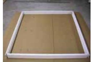
**2** Remove all parts and pieces from the head, sill and jambs. Lay the frame out with the exterior side up, so it will be in the order it is going to be assembled. **NOTE: Make sure center reinforcement on sill does NOT cover the weep hole!**
